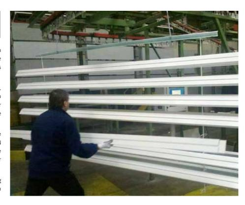
these parts could be painted without additional hand spraying. Not only did this improve the manufacturing cost but improved the lead time immensely as profiles were roll formed at Bridgend and then painted here as well. The photos show the jigging design needed for consistent paint coverage. This was developed over a 3 week period."
